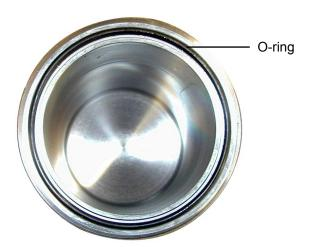
Determine a safe volume and safe initial pressure for the temperature at which the sample will be tested (refer to the chart on page 5). Place the correct volume of fluid into the cell. Be careful not to get fluid in the o-ring groove or on the o-ring.
